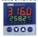
The microprocessor humidity controller on your incubator has two LED displays. The upper display, which is red, represents the actual chamber humidity. The lower display, which is green, represents the target humidity. The controller has 4 buttons marked as follows:
